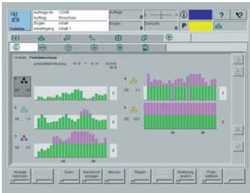
8 Screen shot of the log showing the \Delta E color deviations of all colors.
